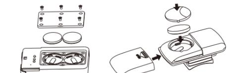
\*Speedometer and cadence sensor battery installation: Open the battery cover on the bottom of the computer with a flathead screwdriver. Install CR2032 battery with positive pole facing battery cover. Replace cover and tighten with screwdriver.
