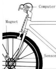
computer in speed mode. Adjust the position of sensor and magnet if there is no or weak reaction.
