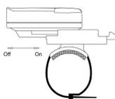
magnet intersects the alignment mark on the sensor transmitter with 1.5mm clearance.
