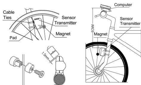
Attach the sensor transmitter to the left fork blade, the distance between computer and the sensor can not exceed 60cm, the closer the batter. Using the shims to adjust the diameter, and using the cable ties(show below) to tie it with the fork. Position the sensor transmitter and magnet as shows, make sure that the arc of the
