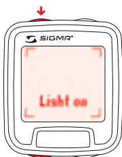
The SIGMA ROX 8.0 is equipped with a light manager. The light can be enabled or disabled (see following illustrations for this). When the light is enabled, the light switches on with every press of a button and stays on for 5 seconds - provided no other button is pressed during these 5 seconds. The display does not change due to using the light.
