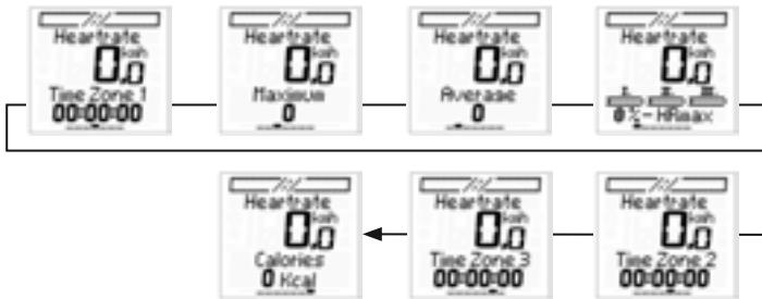
The SIGMA ROX 8.0 has 3 heart rate zones. These zones are calculated automatically when the "user" settings are entered.
