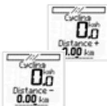
This involves 2 separate distance counters (distance+/distance-). These make it possible to do interval training or a ride following a road map. Both can be pre-programmed, and need to be reset separately from other ride data.
