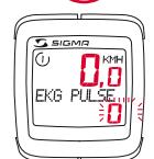
The chest belt transmit some signals (B) ECG PULSE stops to blinking, values are shown.
