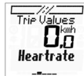
The SIGMA ROX 9.1 has 3 heart rate zones. These zones are calculated automatically when the "user" settings are entered.
