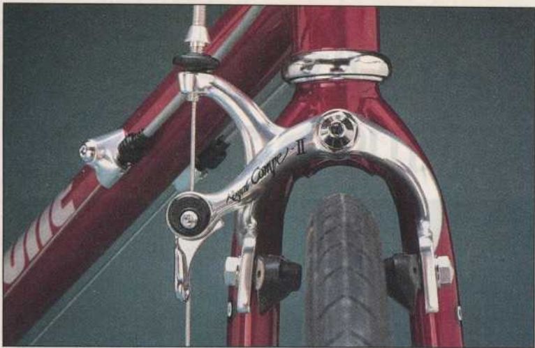
Generous clearances let the RB-2 accept tires much wider than this stock 700x28C, and down-tube cable barrels permit derailleur adjustments while riding.
