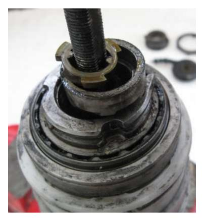
14 - Make a note of orientation, then remove clutch actuator.
