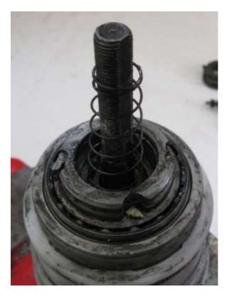
13- Make a note of orientation, then remove clutch and clutch ring. The clutch ring slides along the axle to retract pawls of the left-side pawl ring.
