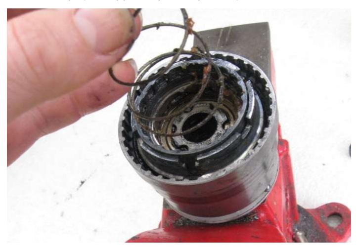
25- Remove planet cage assembly from inside ring gear.
