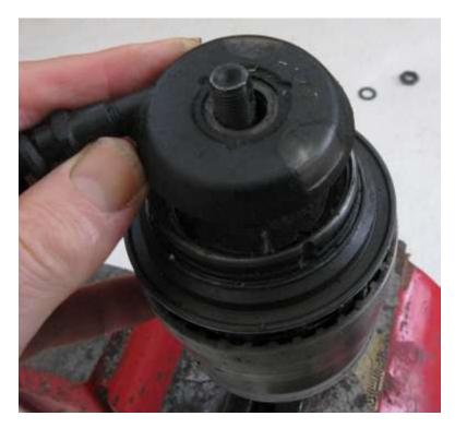
4 - View of right side of hub after pulley/bearing cone assembly has been removed. The driver is now exposed. The rightside smaller bearing cup is visible, just inside the 3-lug fitting for the sprocket. David had already disassembled the hub this far, and the bearing retainer which belongs here is absent.
