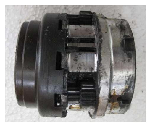
27 - Remove ratchet ring from inside planet cage. The six lugs at the inside of the narrower end of the ratchet ring engage the sun-gear assembly as shown in step 24.
