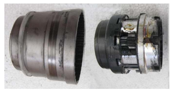
26 - Pry inner ring gear (at left) from planet-cage assembly with a flat-blade screwdriver, if necessary.
