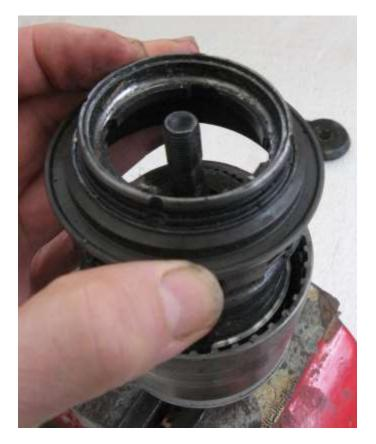
6 - Remove dog ring. The teeth on its inner face are a ratchet for pawls, not a ring gear. The lugs engage the planet cage (see step 24).
