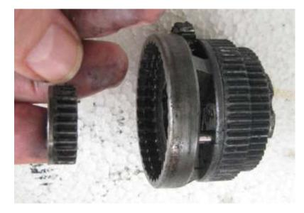
30 - These are the sun gears and associated parts of the assembly shown in the previous photo, disassembled (photo credit: Aaron Goss). The circlip (left) might be damaged during removal, so you might skip this step.
