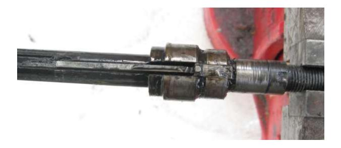
23 - I've lifted up the key and slid the rod to the left to show how they may be removed. Note: the rod had been replaced in position and is upside down. The end which attaches to the key should be farther from the centerline of the axle.
