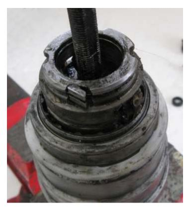
16 – The pawl ring has four sets of pawls. The leftmost set, already described, drives forward and the other three sets are driven forward.
