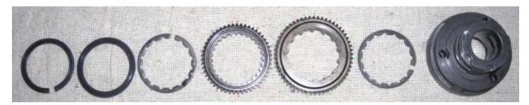
31- Same assembly, further disassembled. The four small internal pawls are inserted with the peak in the middle facing outwards (engaging the teeth inside the two gears). The larger end of each pawl is clockwise in the image above and counterclockwise in the images below. The pawls are of two types: relieved sides inside the bore face each other. (left photo credit: Aaron Goss).
