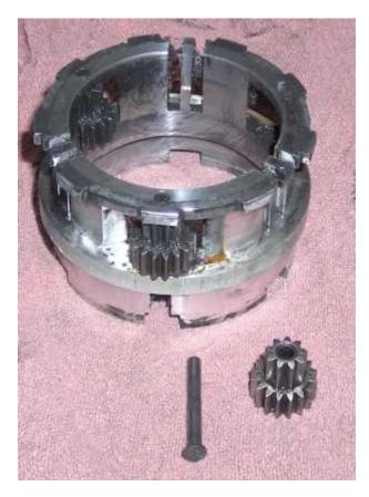
27- Separate inner ring gear from planet gears in sun-gear assembly. Now we see what seized this hub. Wider/narrower increase or decrease ratios depend on which of three sun gears is engaged. Two of them, visible in this photo, may be engaged or disengaged; the remaining one, shown in the next photo, is constantly engaged..
