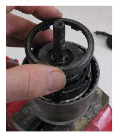
7 - Remove right-side pawl ring. The four cylindrical protrusions mate with the driver, and the pawls engage the dog ring.
