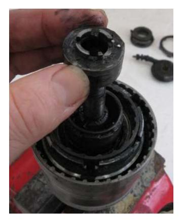
9 - Now I have turned the hub over and we are looking at the left side. A pawl and a pawl spring are missing, but one pawl remains, oriented to drive the wheel by engaging the ratchet inside the left end of the hub shell. The two narrower recesses at 90 degrees to the pawls probably engage the coaster brake mechanism in the coaster-brake version.
