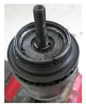
5 - Remove driver. The cone race of the larger right bearing is on the underside of the driver, not visible in this photo. The cup for that bearing is press-fit into the hub shell.
