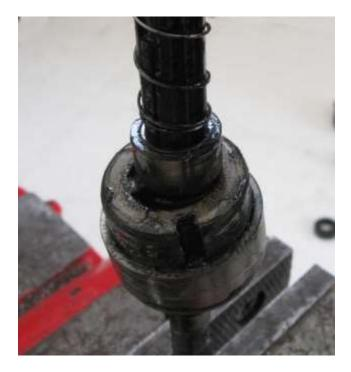
19 – Spring and shifter parts are now removed from the axle.
