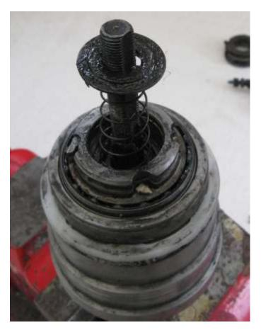
12 - Remove spring. Notice that it is conical, with the larger end toward the middle of the hub.
