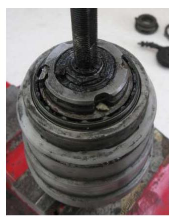
10 - Remove crush nut. This nut is deformed during assembly to prevent it from unscrewing. Replacements are available from Aaron's Bicycle Repair, <u>http://rideyourbike.com</u>. Or send your hub to Aaron, as he has a stock of hubs to cannibalize and can do an expert repair.
