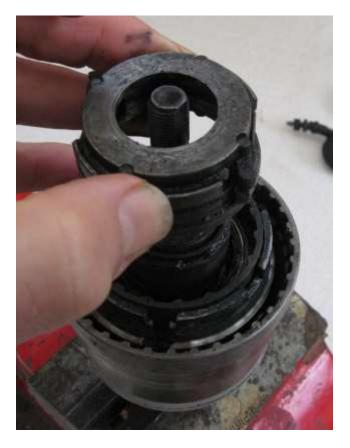
8 - Remove shifter cam. The right side of the cam engages the pulley of the pulley/bearing cone assembly. One of the four lugs is cut away to make room for a small spring on the back of the pulley where lugs engage the cam. The left side of the cam pushes parts inside the hub leftward to shift gears. Orientation of the cam matters. Make a note of it.
