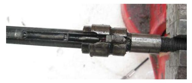
22 – Shifter parts on the opposite face of the axle. Note: the rod had been replaced in position and is upside down. The end which attaches to the key should be farther from the centerline of the axle.
