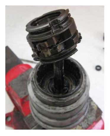
17 - These are the parts which have been removed from the left end of the axle, in order right to left, and left side up (photo credit, Aaron Goss). The left-side shifter parts engage and disengage sun gears to provide wider and narrower ratios – both increase and decrease ratios, which are the inverse of each other.
