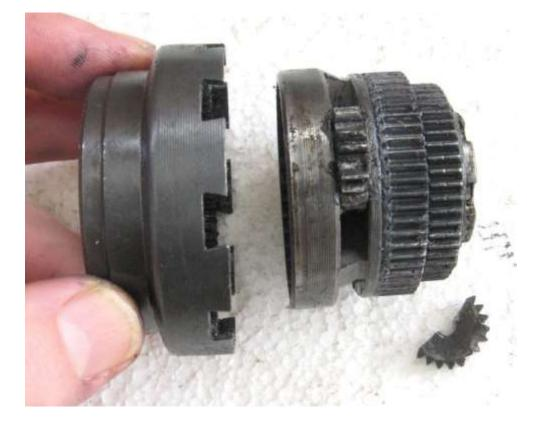
29 – Remove small sun gear from inside planet gears. This frees the pawl pins for the internal pawls – they could fall out.
