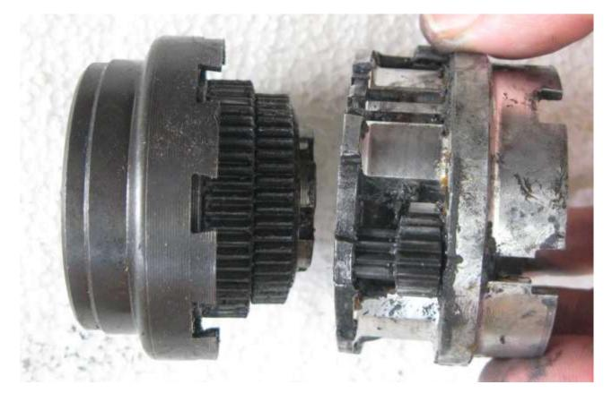
29 -Pinion and pinion pin removed from the planet cage (photo credit: Aaron Goss).
