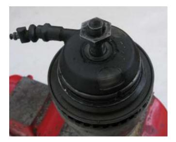
2 - Remove washer. This will come off along with the pulley/ bearing cone assembly if not removed separately.
