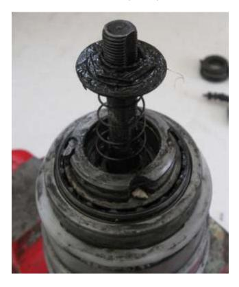
11 - Remove two washers. There is a washer with internal tabs on top of the larger one (The washers are stuck together with grease in this photo). I disassembled the hub dirty because grease kept some parts, like the one pawl here, from falling out, and so I could still determine where they belonged! Method to my madness...
