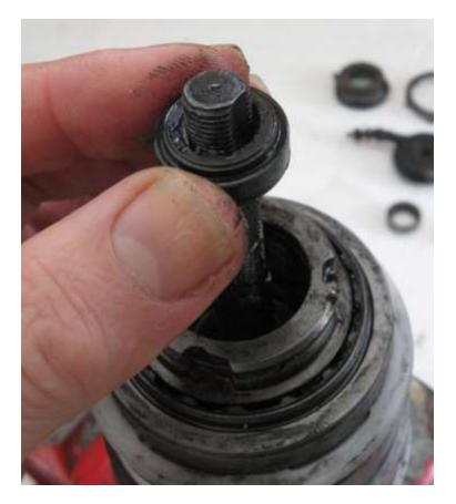
15 - Remove left-side pawl ring. As noted earlier, a pawl and the pawl spring are missing. These pawls drive the wheel in all of the hub's ratios. The coaster-brake version of the hub would probably have parts engaging the two unused, narrower recesses at 90 degrees from the pawls.
