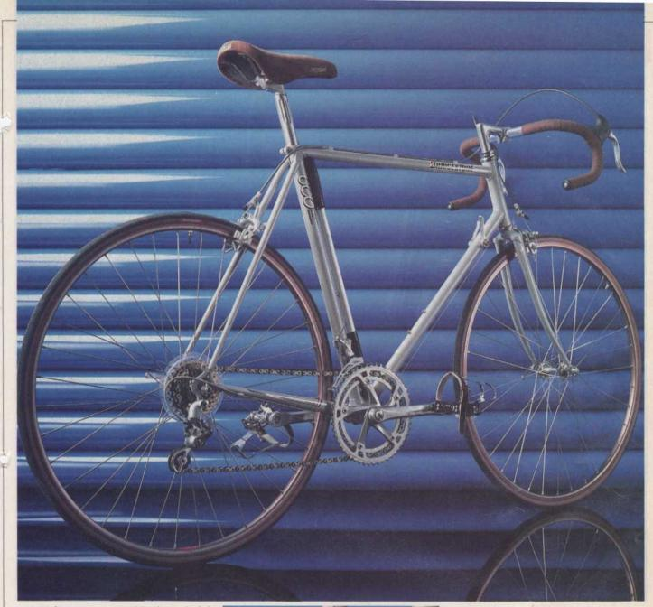
The \$370 Bridgestone 600 (above) proved a little skittish in high-speed descents, a trade-off for its excellent low-speed maneuverability. Silver-gray paint is accented by the rich brown saddle and handlebar tape. Self-centering brakes on the Bridgestone (right) make rubbing brake shoes a thing of the past—a boon for cyclists who would rather ride than work on their bikes.
